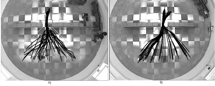
Fig. 2. a) Robot trajectories under manual control (39 runs, training data). b) Trajectories taken under model control (41 runs, test data). The white lines on the floor were used to aid the human operator in selecting start locations, they were invisible to the robot.
